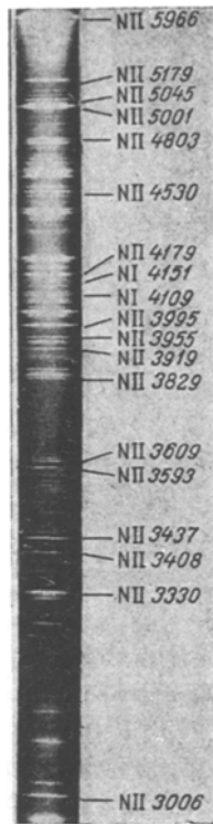
Fig. 1. Emission spectrum of plasma jet, I = 200 A, U = 165 V, R_g = 50 liters/min, d_c = 2.5 mm.
